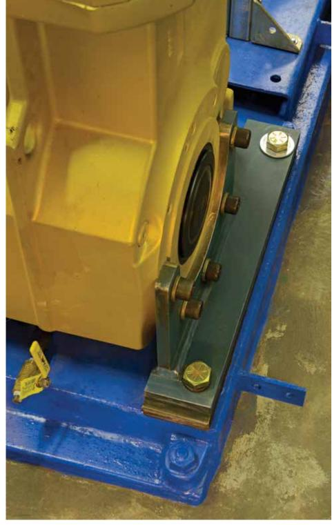
Since the Quantis Gold package needed to be installed in the same spot where the old drives sat, Baldor was able to provide fabricated steel brackets, which made the installation quick and easy. Plant officials say the solution Baldor provided made the Quantis Gold package a simple drop-in replacement.
